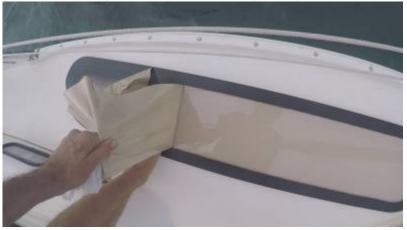
After sending the window edges, and cleaning with mineral spirits, I applied the 3M VHB tape along the perimeter of the window.
