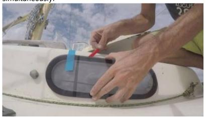
Once the windows were firmly held in place with the VHB tape, I carefully masked out about 1/4« from the perimeter of the window so that I would have a nice edge after the sealant was applied.
