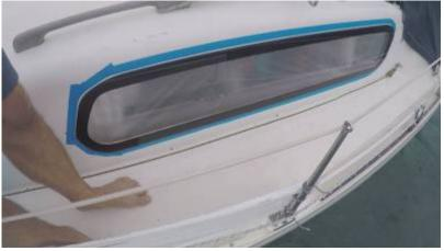
I used Dow-Corning 795 sealant, which is also structural. To make sure I filled the gap between the window and hull, I used a syringe.
