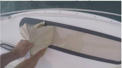
After sending the window edges, and cleaning with mineral spirits, I applied the 3M VHB tape along the perimeter of the window.
