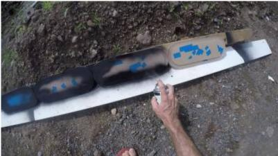
Pealing off the protective paper after painting, and just prior to installing. Leave it on as long as possible, as acrylic scratches relatively easily.
