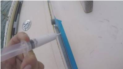
Make sure you remove the masking tape before the sealant cures, and preferably immediately after application.
