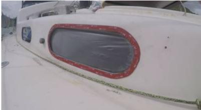
This is the tricky part. The method I used was to pull the red protective film on the VHB tape just
