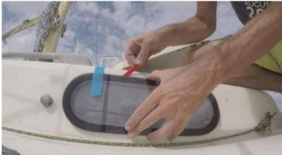
Once the windows were firmly held in place with the VHB tape, I carefully masked out about 1/4« from the perimeter of the window so that I would have a nice edge after the sealant was applied.
