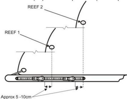
The position of the sliders on the track can be adjusted during a sail trial. The two plastic end caps can now be fitted, ensuring they locate over the end on the track. (This is a push fit) use the centre punch to mark position then remove before drilling and tapping as previously stated.
