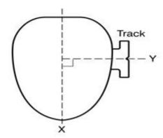
Remove track, drill using 4mm drill and tap using M5 tap then secure in position using M5 machine screw.
