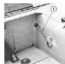
Fig. 14 1. Throttle lever for engine throttle and propeller pitch.
