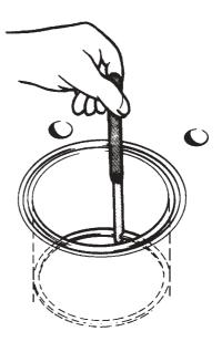
Fig. 41. Checking of piston ring gap
